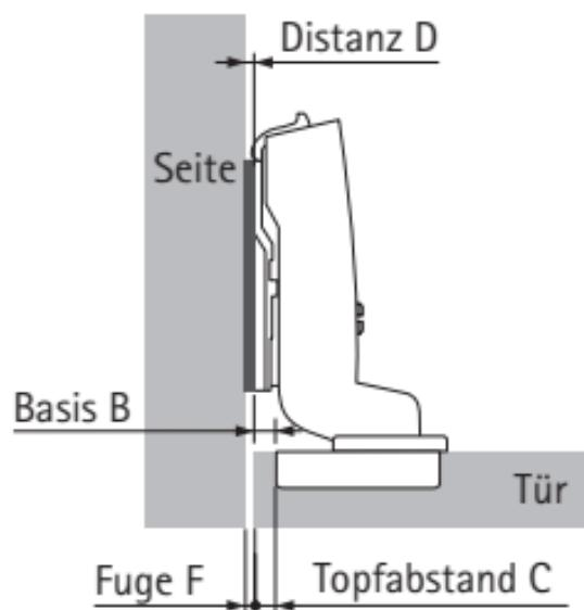
$$\begin{aligned} \text{Distanz D} &= C + B + F \\ &= \text{Topfabstand C} - 4 \text{ mm} + \text{Fuge F} \end{aligned}$$
