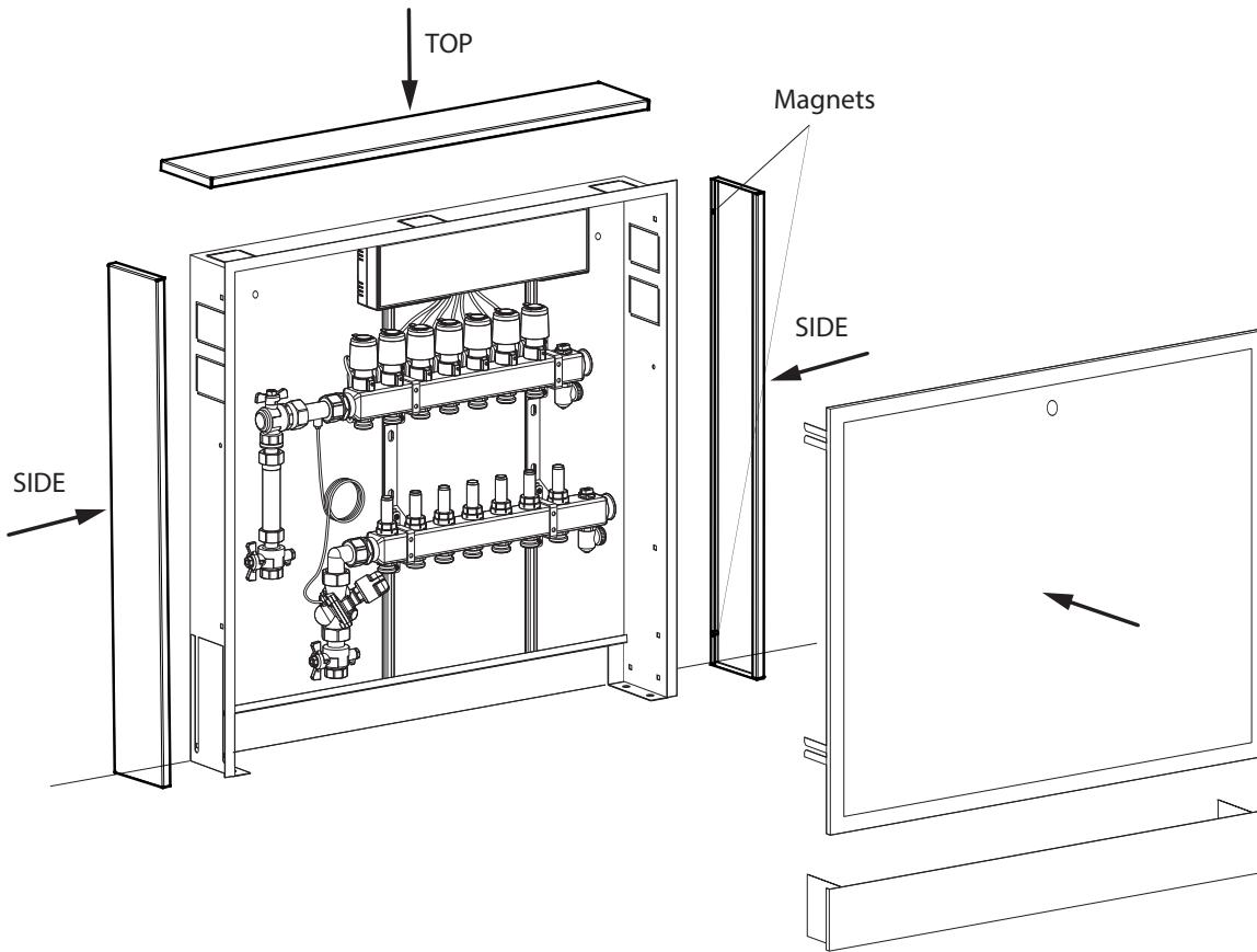
When mounted on wall the cabinet needs to be mounted floor standing!
